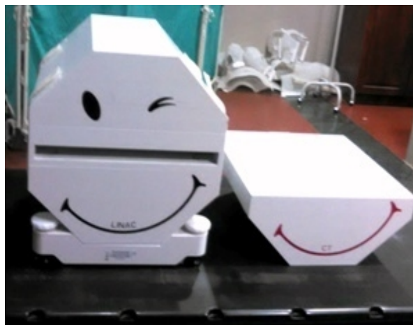
FIG. 2: Octavius phantom set (LINAC phantom and CT phantom).
