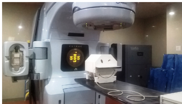
FIG. 1: Experimental Set-up for the pre treatment quality assurance tests for IMRT. PTW 2D ionization chamber array inserted inside the Octavius CT phantom, SSD was kept at 84 cm.
